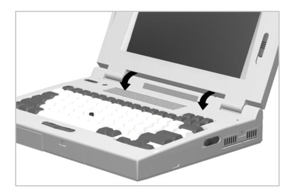
Figure 5-23. Removing the CPU Cover
